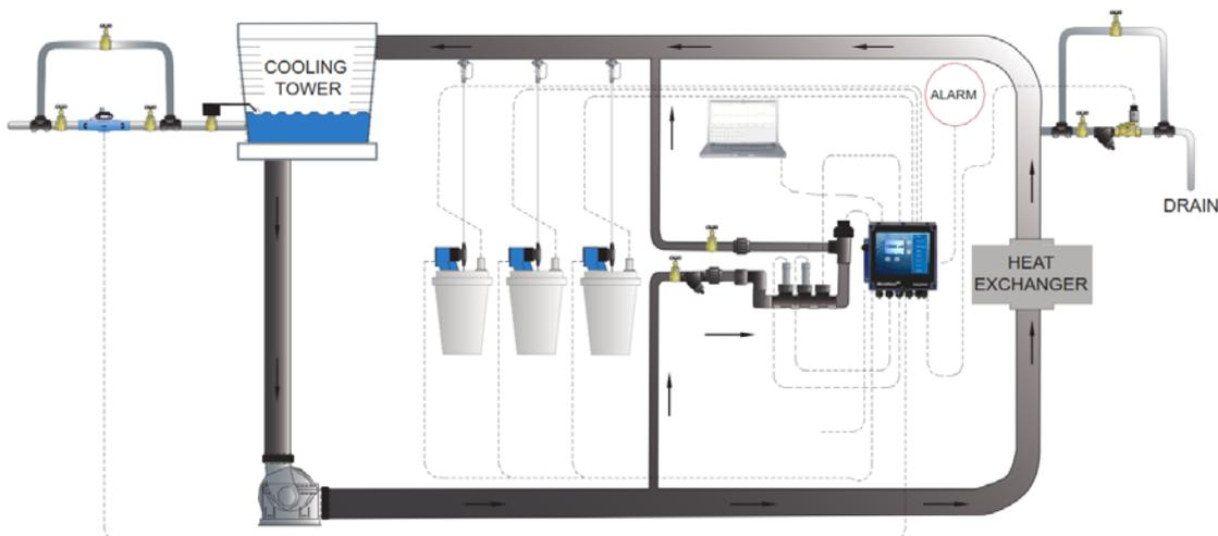
**⚠** Over pressurization of the plumbing can occur when cooling tower is higher than the piping and controller system. Ensure all pressures have been accounted for. Verify piping and sensor allowable temperatures are above maximum temperatures of the system.
